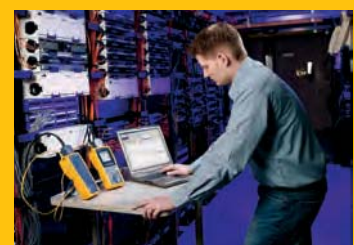
DTX-1800 with DTX 10 Gig Kit to test Alien Crosstalk performance
